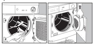
The filter in the inner door must be removed for cleaning.
